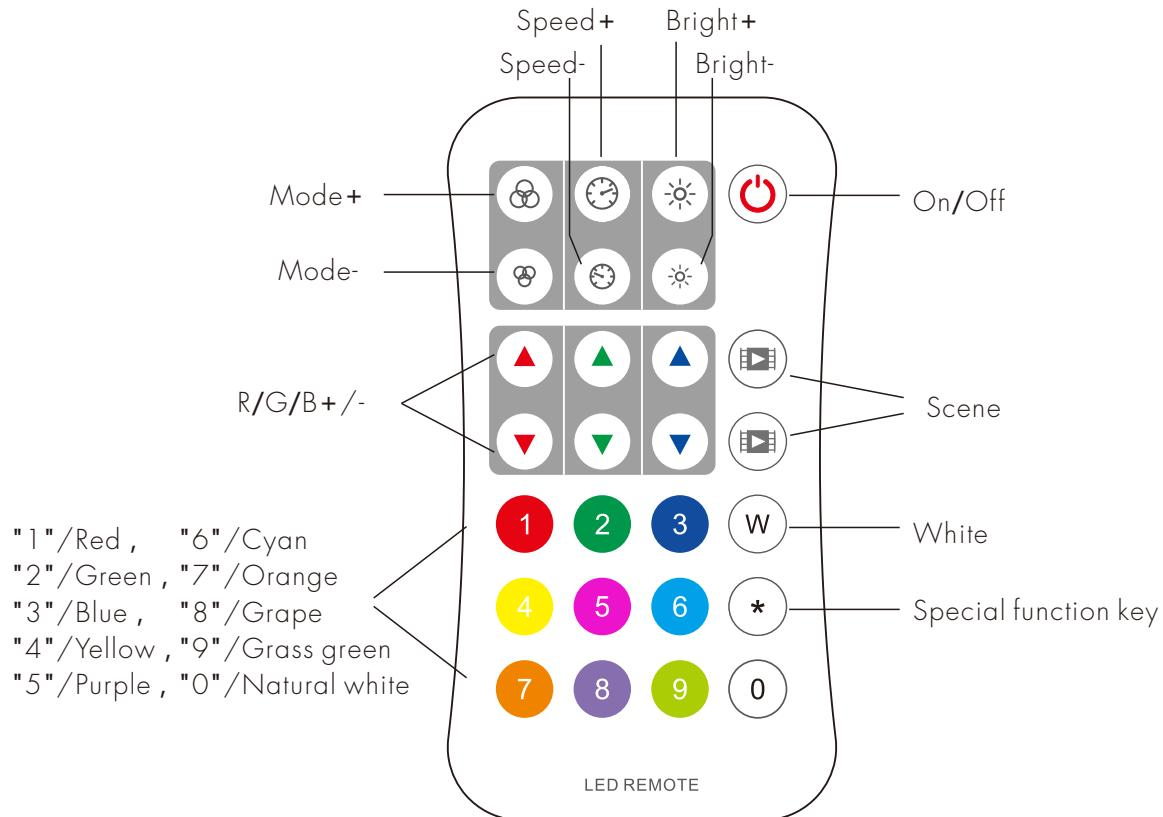
**Mode+/-:** Short press switch dynamic mode built in controller, long press 2s Mode+ run mode cycle, long press 2s Mode- run the first mode.
