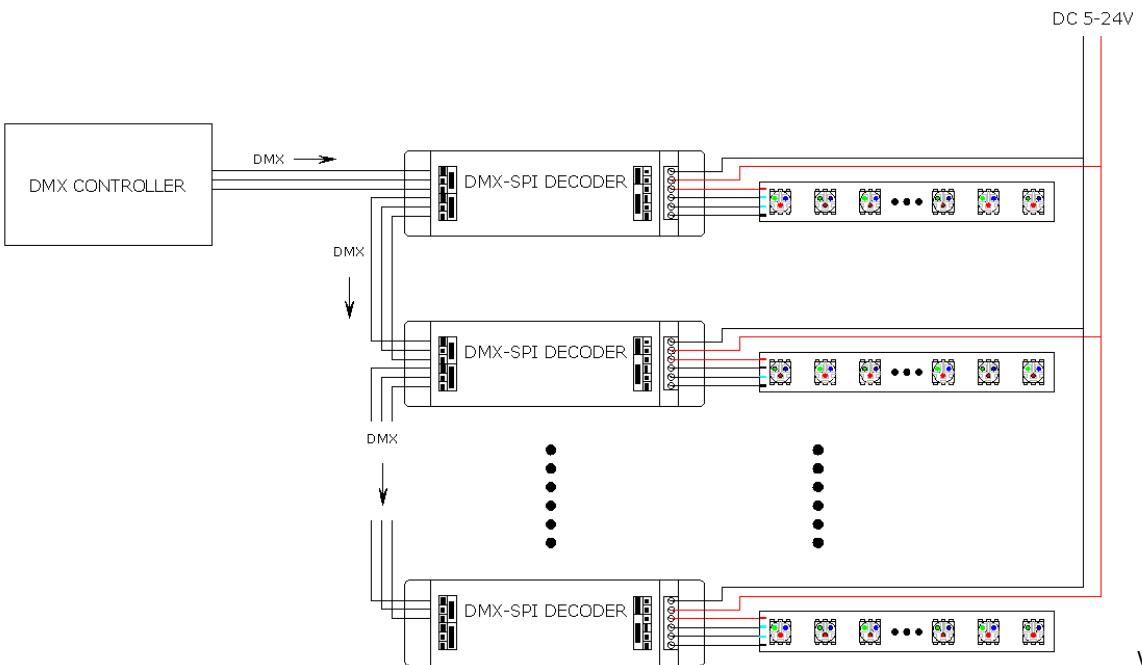
**Double power connect single signal line strip condition:** if the V+ voltage 玆界 狹玲赫惋漫 楊紗 淚繫玲 玲梔攀 紗愀洩攀 明梔玲梔 振繫淚玲赫繫斃斃攀赫 楊淚漫珎玲 紗繫斃玲愀最攀 楊淚換 light signal is single, you need to connect another power supply.
