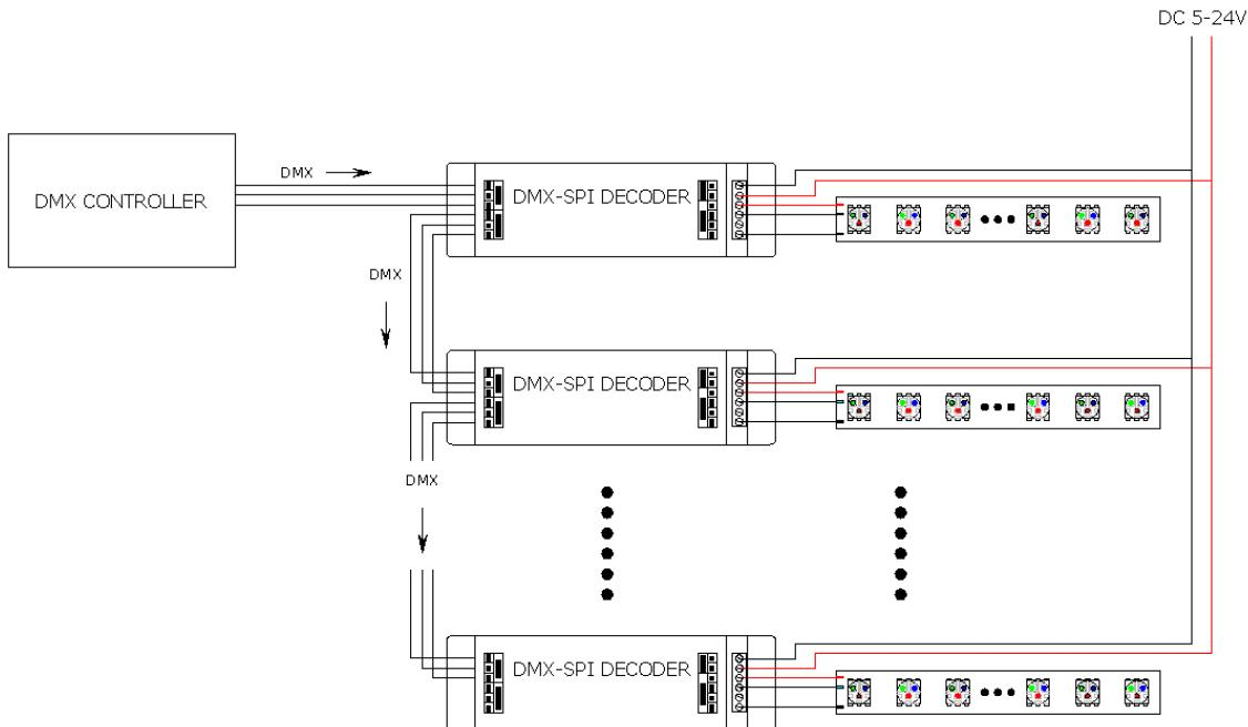
**Single power connect double signal line strip condition:** if the V+ voltage of strip is the same with controller input voltage, and the light signal is double then it can directly connect with the controller V+;
