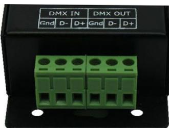
**DMX IN:** input interface of DMX signal, D+ should be connected with positive of signal, D- connected with negative of signal, Gnd connected with ground.
